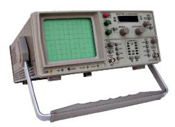
Spectrum Analyzer is used for the early test in the development of electrical products, troubleshooting of CATV/MATV system as well as the test and trouble diagnosis of cellular phone/paging system.
