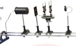
ME 854 - To find the specific rotation of sugar solution by using a polarimeter
