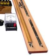
ME 847 - To determine the Frequency of A.C. Mains using an Electric Vibrator.
