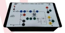
Instruments provided with 220V AC power supply, Lamp holder, intensity control Potentiometer.
