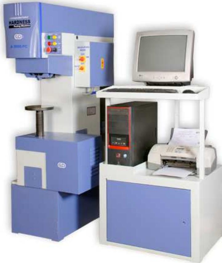
Design of machine is similar to OPFB-A, However with Computerized measurement of Brinell impression. Machine confirm to IS 2281/2005, BS 240 & ASTM E-10.
