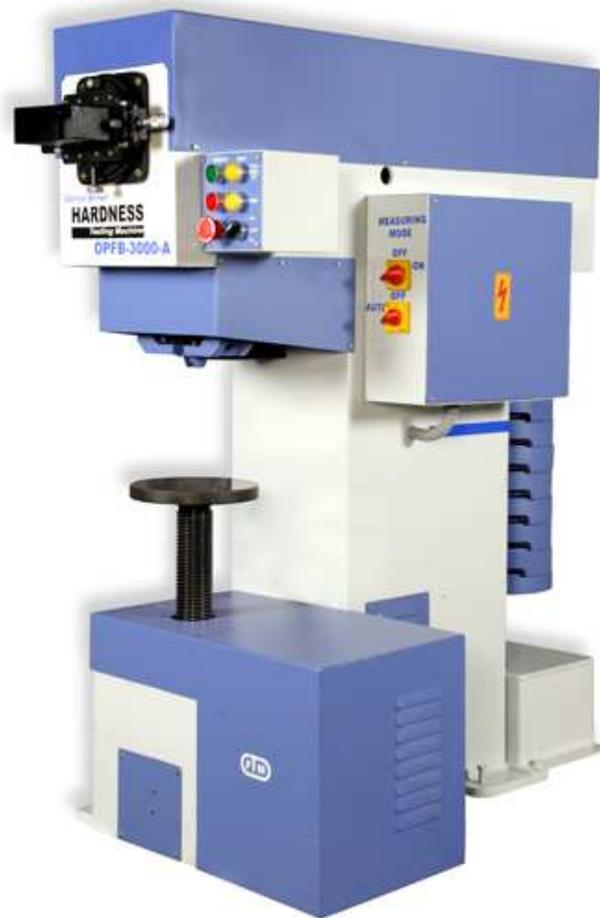
Machine designed with fully automatic loading, measuring and unloading cycle. A compact hydraulic power pack and control circuit with built in optical device with 14X magnification provided in front to project diameter of ball impression on glass screen with micrometer measuring system with 0.01 mm least count.
