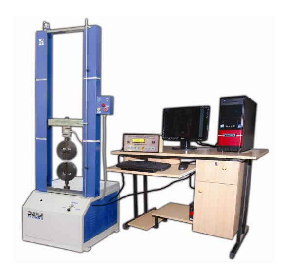
These models are suitable for testing metals and iron, Plastics, Rubber, Ceramics, Fabrics , Composites, Cables and wires.
