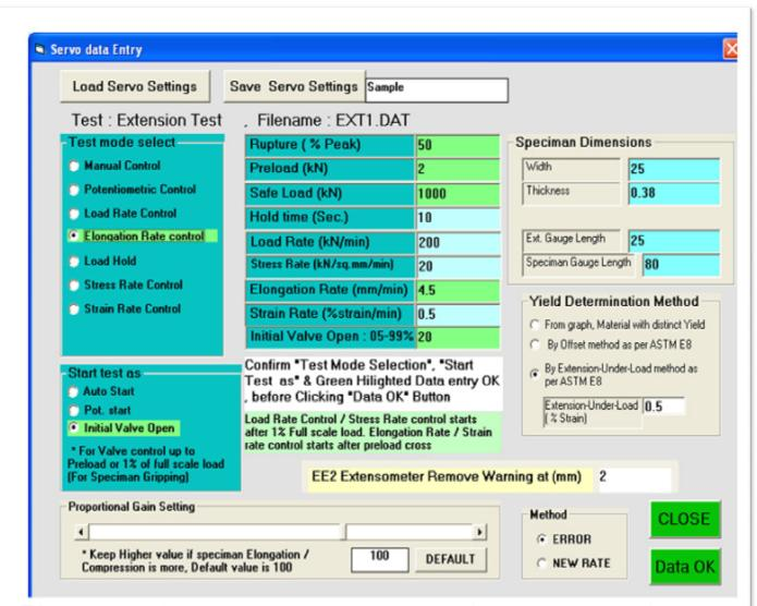
This screen opens when you start "Servo Test" from main menu. (For Servo Controlled m/c)
